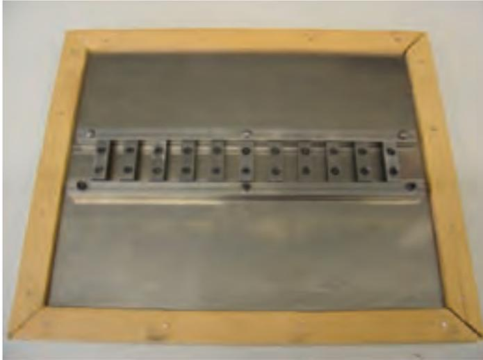
Figure 7 - Mould for preparing SIC test specimen
